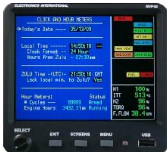
The “#Cycles” can be setup to count airframe (takeoff/landing) cycles or engine start cycles. The value of “#Cycles” is based N1. When a preset high value of N1 is reached the “Status” field will display “Armed.” Then, when a preset low value of N1 is reached the “Status” field will display nothing and the value of “#Cycles” will be incremented by one.
