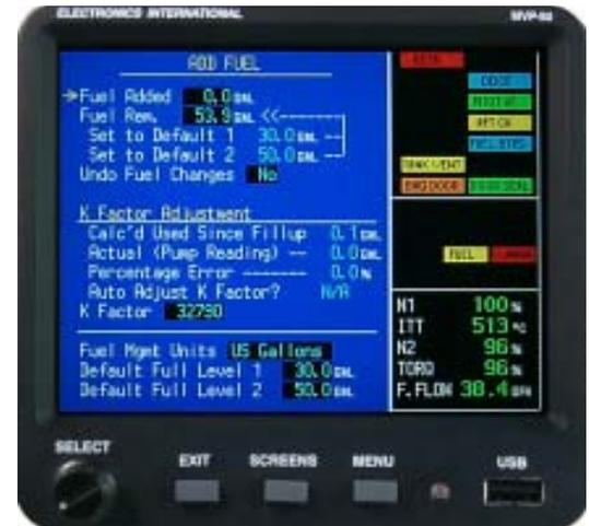
the K Factor. The K Factor is a measurement of the pulses per gallon that the flow transducer outputs. Due to variations in the installation of the flow transducer, it may be necessary to adjust the K Factor for the first few flights in order to get an accurate fuel remaining, fuel used and flow reading.
