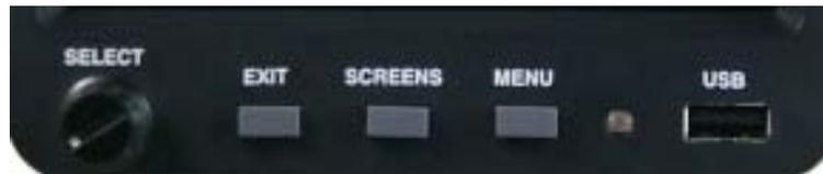
**EXIT Button:** Pressing the EXIT button will exit you out of a specific operation. Repeated presses will exit you out of the current screen, returning you to the previous screen viewed. You can always return to the Main Engine Instrument Screen by *repeatedly* pressing the EXIT button.
