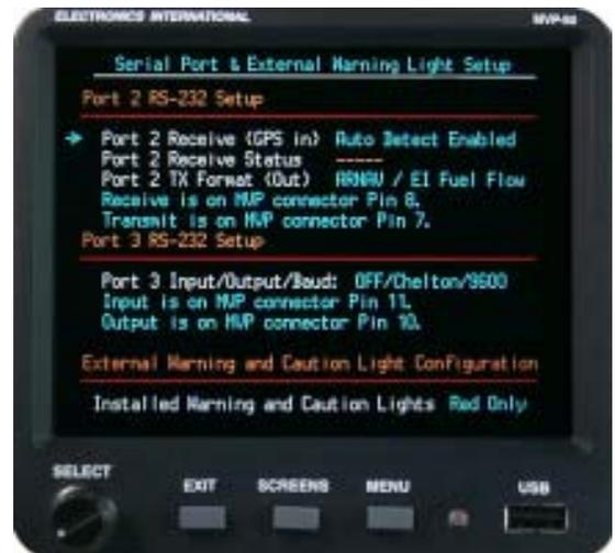
**“Port 2 Receive Status”:** When the Port 2 Receive field is set to “Auto Detect Enabled” the Port 2 Receive Status field will show one of the following:
