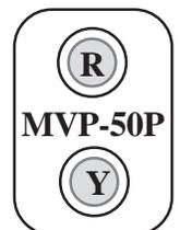
Pushing any button, or rotating or pushing the Select knob when the Caution or Warning Light is blinking will acknowledge the blinking and the blinking will stop. Also, acknowledging a voice warning using the external “Voice Alarm Control Panel” will stop the blinking of the Caution and Warning Lights.
