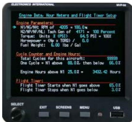
**“One Cycle = N1 above \_\_\_\_\_% then below \_\_\_\_\_%”:** This line allows you to set the logic to determine when a cycle is counted (engine or flight). An engine cycle is counted for each engine start. To record engine cycles, set the **“N1 above”** field to a value just above the maximum N1 that can be reached during start with no fuel (around 35%). Set the **“then below”** field to a very low value (around 3%).
