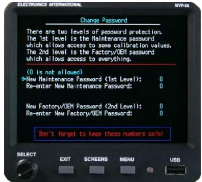
**6.1.1 Level #1 Password (Maintenance):** The Level #1 password is for the installer or maintenance personnel. This password allows the installer to perform the following:
