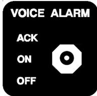
The Voice Alarm Control Panel is an external panel used to control the voice warnings provided by the MVP. The MVP voice warning system is a powerful system that provides an immediate and intelligent audible warning regardless of the pilot’s head position or focus. The instant an operating level of any function reaches a red and/or yellow operating limit, a chime will sound in the headset and a pleasant female voice will announce a phrase, such as: “Check Oil Pressure,” or “Check Fuel Pressure.”
