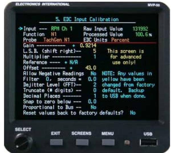
**“Reference:”** The Interim Value may be referenced to another Function. The value of the Function selected in this field will be added (+) or subtracted (-) from the Interim Value. Differential measurements can be made by subtracting one Function from another. Temperature measurements based on thermocouple probes must be temperature compensated by referencing the “T. COMP” (temperature compensation) Function.
