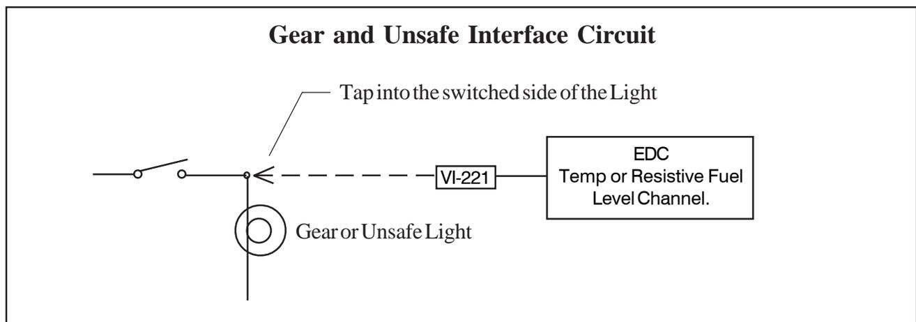
There are three options for interfacing the EDC to the aircraft’s gear system.
