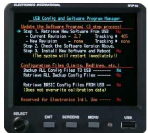
The “Retrieve ALL Backup Config Files” command reads all the stored configuration data on the USB Data Stick. If the configuration data was NOT stored to the USB Data Stick by same MVP that is retrieving it, the command will fail and an appropriate message will be displayed. Each MVP system has the following unique calibration data that should not be shared with other MVP systems:
