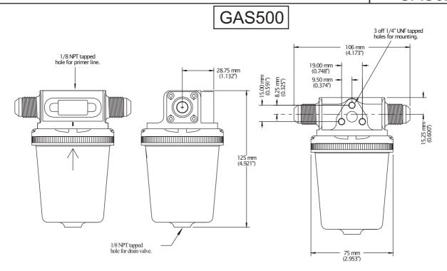
Suitable for engines of 500+ HP, the GAS500 is a tough, rugged and compact Gascolator. Precision machined from aircraft grade Aluminium and chromic anodised for protection, this Gascolator is the leader of the field.
