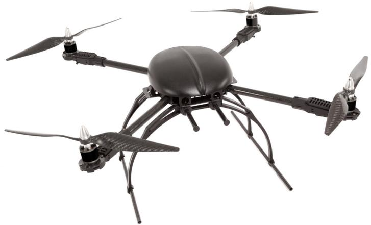
Figure 2-5. Common quadcopter type multirotor.
