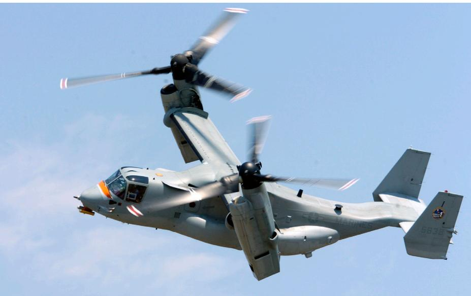
Figure 2-6. Osprey tilt rotor aircraft transitioning to forward flight.
