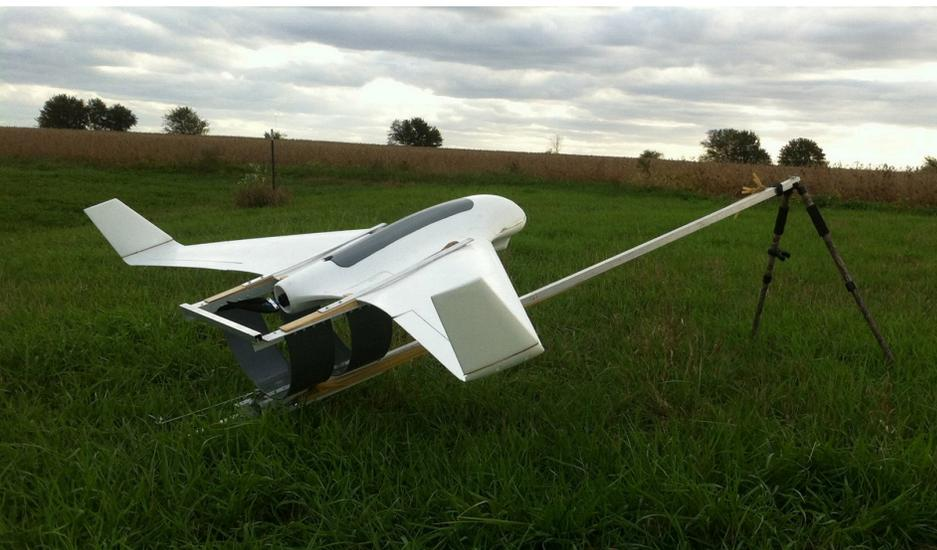
Figure 2-4. A catapult may be used in the absence of a suitable runway for takeoff.
