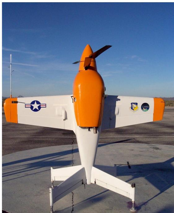
Figure 2-8. Takeoff and landing position of tail siter unmanned aircraft.
