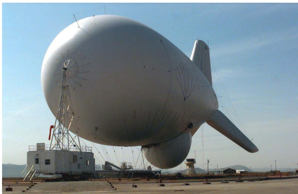
Figure 2-10. An aerostat type airship with tethering tower.
