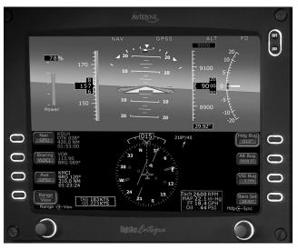
Figure 2-2. A typical primary flight display (PFD)
