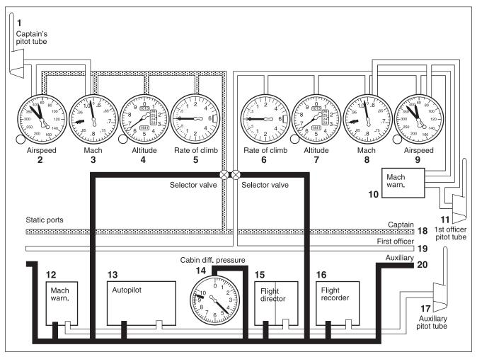
Figure 2-1. Typical pitot-static system
