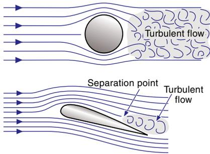
**Figure 1-10** Turbulent flow.
