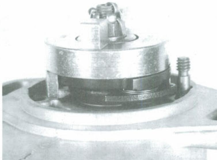
**Figure 19.** Flyweight heel strikes stop pin, disengaging flyweight from stop pin. Impulse coupling spring spins magneto.
