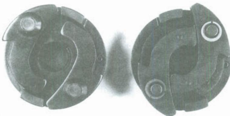
**Figure 17.** Impulse couplings. Old style on left, new style (per service bulletin 599D) on right.
