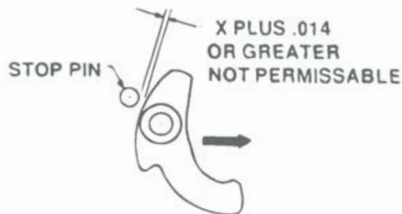
**Figure 20.** Bendix flyweight axil wear check. Too much wear, and the heal of the flyweight hits the stop pin causing the toe to engage the next stop pin.
