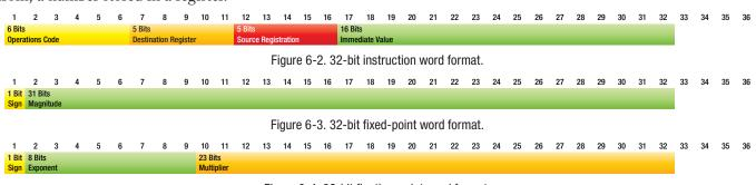
Figure 6-4. 32-bit floating-point word format.
