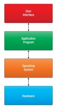
Figure 6-5. Application programs run on top of the operating system.
