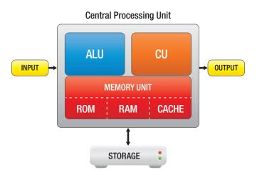
Figure 6-7. Components of the Central Processing Unit.
