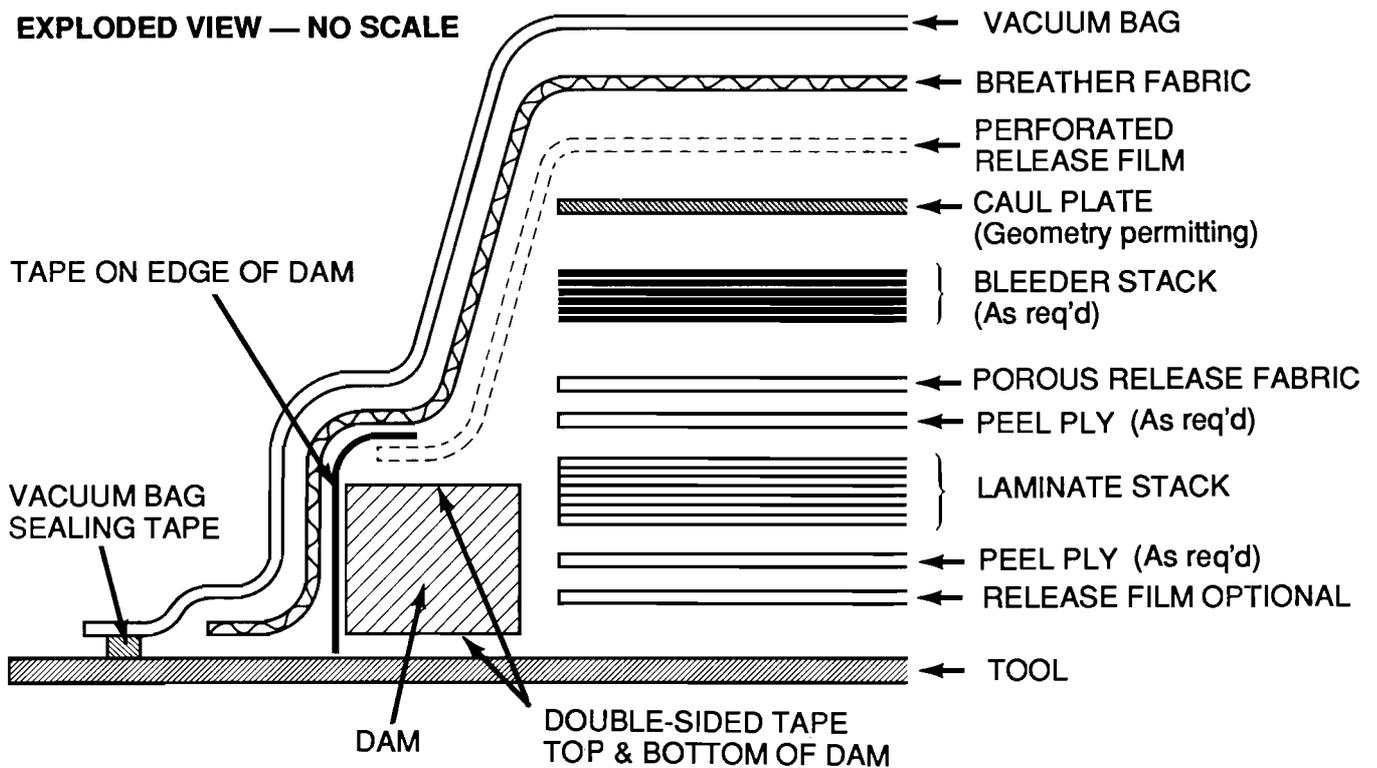
Figure 7-6. Typical layup used for a complex carbon fiber-based part.
