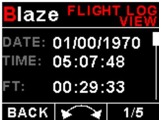
Use the rotary control to view the next flight log entry.
