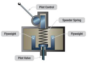
Figure 17-23. Governor sensing an on-speed condition.
