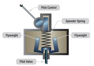
Figure 17-21. Governor sensing an underspeed condition.
