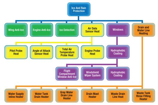
Figure 12-3. Ice and rain protection systems on a large transport aircraft.
