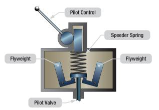
Figure 17-22. Governor sensing an overspeed condition.
