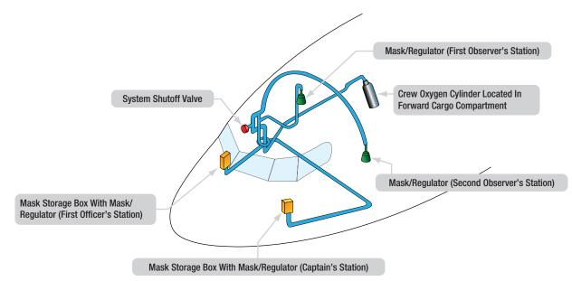
Figure 11-14. Location of demand-flow oxygen components on a transport category aircraft.
