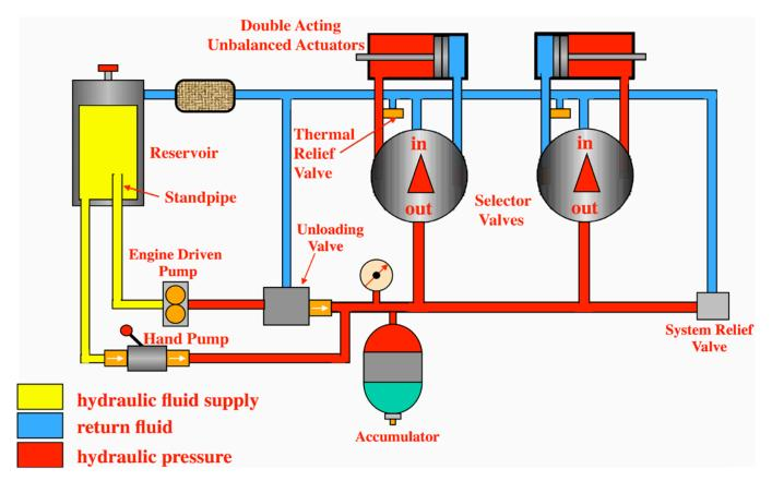
Figure 7-12. Small airplane hydraulic system.
