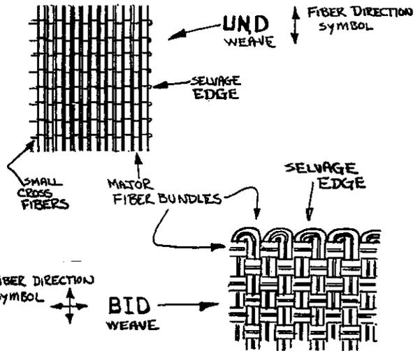
BID is generally used as pieces which are cut at a 45° angle to the selvage and laid into contours with very little effort. BID is often applied at 45° orientation to obtain a desired torsional or shear stiffness. UND is used in areas where the primary loads are in one direction and maximum efficiency is required, such as the wing skins and spar caps. Correct orientation of fibers is extremely important.
