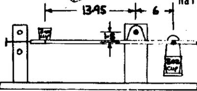
Safe-T-Poxy resin to hardner ration is 100 parts to 43 parts by weight. By volume it is 7 parts resin to 3 parts hardner.
