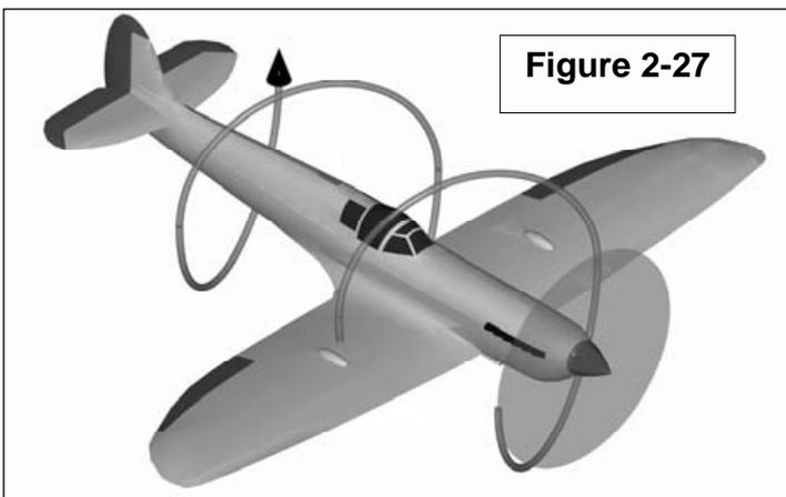
The magnitude and effect of the spiraling slipstream varies greatly between aircraft designs, as such, no easy rules of thumb can be provided to isolate these forces from other propeller phenomenon. It is the result of the air circulating around the aircraft because the propeller imparts such motion to it (Figure 2-27).
