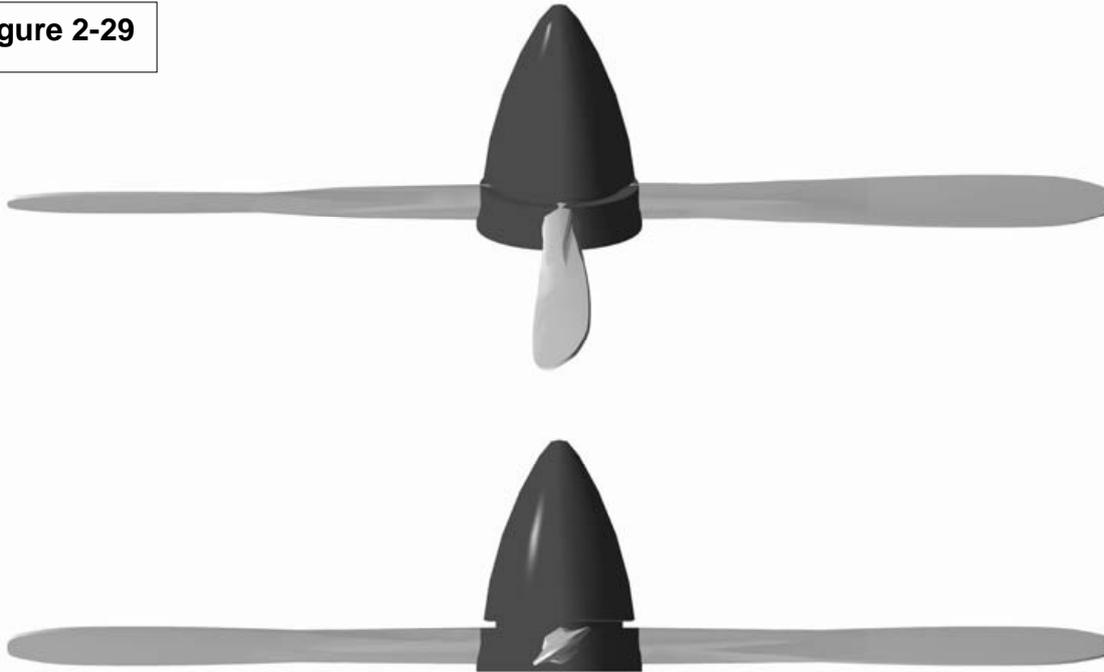
The reaction to this is a left yaw of the aircraft (for a prop which rotates clockwise as viewed from the rear) because the thrust being produced on the right side of the aircraft (down going blade) is about twice as much as the up going blade on the left side (Figure 2-30) (the converse effect is that if an aircraft is flying in slightly yawed flight, a pitching moment is produced).
