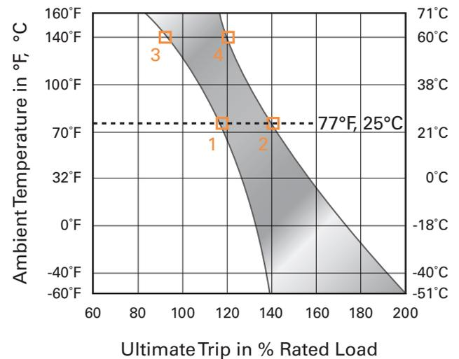
Performance characteristics are based on room temperature (77°F, 25°C). Consult Derating curve for ambient temperatures significantly higher or lower than standard room temperature.
